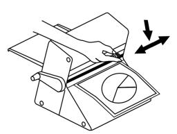
Step 3 - Trim to desired length using the cut blade at the roller exit. Apply pressure down on the orange blade holder and slide to the left or right.
